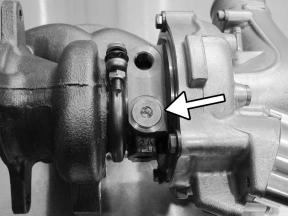
on the inside of the turbocharger (the side that faces the engine), confirm that the plug is in the bottom location:
