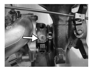
2) The DV should be oriented so that the electrical connection is facing up and forward (toward the engine). Install the longer supplied bolt in hole most opposite from the electrical connection.
