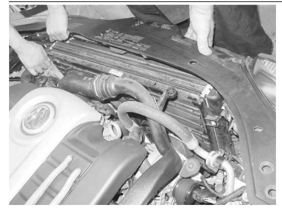
23) With a partner, remove the two APR-supplied bolts from both sides of the radiator core support. Remove the condenser/intercooler/radiator/fan assembly from the core support by sliding the upper part of the intercooler assembly away from the top of core support. While doing this, the intercooler side grommets will side out of the core support. Once the side grommets of the intercooler are free, lift the intercooler assembly up and out of the core support. Set the core support aside.
