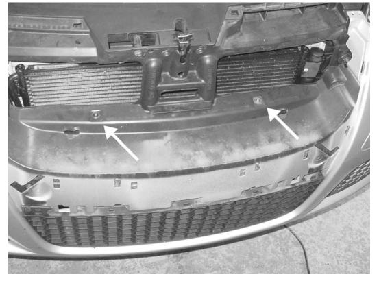
7) Remove the two T25 Torx Screws and the two T30 Torx Screws on the top of the bumper that were revealed when the radiator grill was removed.
