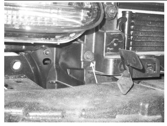
19) Loosen the T30 screws that connect the radiator core support to the intercooler side grommets. There is one screw on either side that is revealed once the headlight support is removed.
