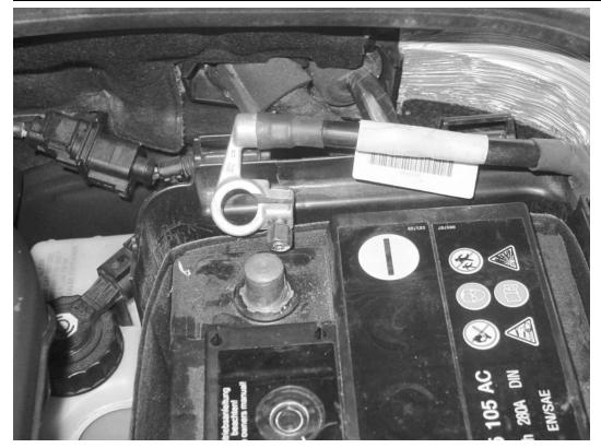
1) Support the car on jack stands or a lift. Open the hood and disconnect the 10mm negative battery terminal.
