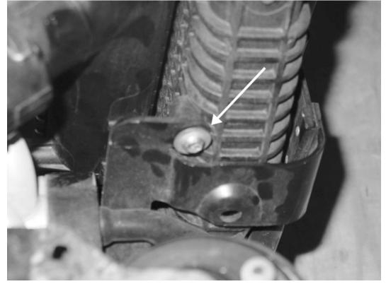
25) Begin to separate the A/C condenser from the intercooler by removing the four T30 screws from the front of the condenser. There is also one T30 screw on the passenger side holding the condenser lines to the intercooler. These five screws are not reused.
