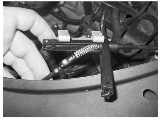
11) Unclip the hood release coupling located above the driver's side headlight. Open the coupling with a small screwdriver and release the cable.
