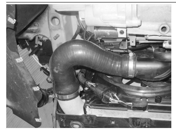
43) Install the APR driver's side intercooler hose with the supplied hose clamps.
