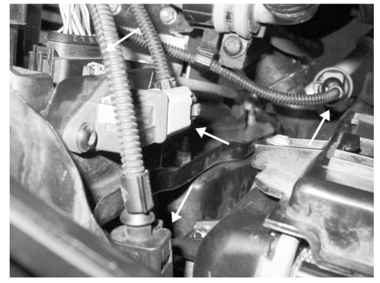
37) From the top of the car, reconnect the following electrical connectors: A/C pressure sensor, both headlights, and the hood latch Again, after confirming sensor. the battery on the car is still disconnected, reconnect both of the yellow airbag crash sensors.
