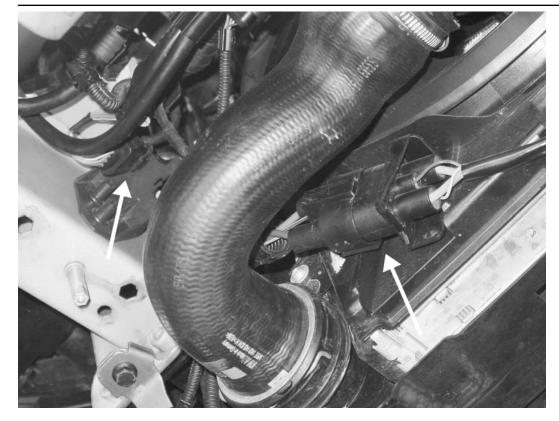
17) From below, disconnect the fan wiring harness connector located on the back of the driver's side of the radiator fans. On the driver's side frame rail, some models have a connector to disconnect the wiring harness that goes to the foglights and sidemarkers. Otherwise it is necessary to remove the wiring harness from the radiator core support, including the outside air temperature sensor.
