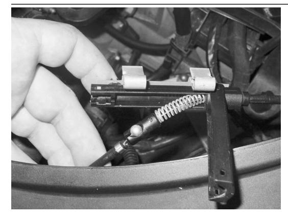
47) Reconnect the hood release cable and reconnect the housing with the factory clips behind the drives side headlight. Confirm that the hood release works from inside the car before closing the hood.
