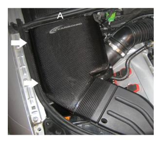
Also note: There is a rubber fuel injection hose that passes over the MAF and exits the airbox out a hole in the front of the box. Be sure to route this hose without any kinks or bends.
